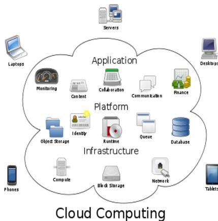
Figure a Architecture of cloud computing
