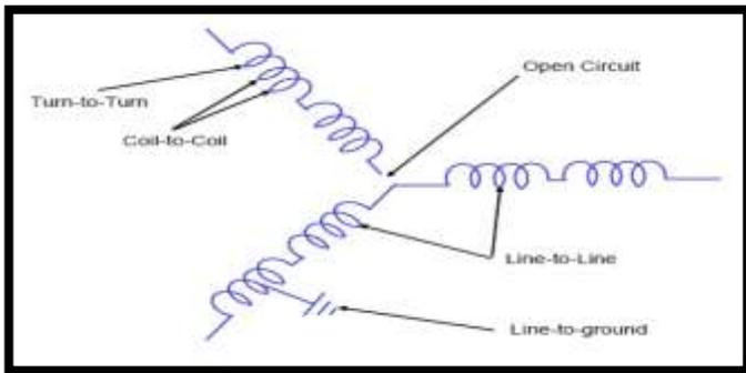
Figure 2: Different short and open stator winding turn faults
