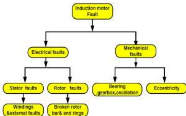
Figure 1: Fault classification in induction motors
