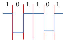
Fig.3. NRZ coding example
