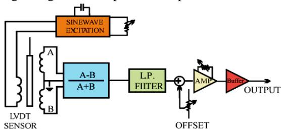
Fig 4: LVDT Based Digital Weighing System [9]
