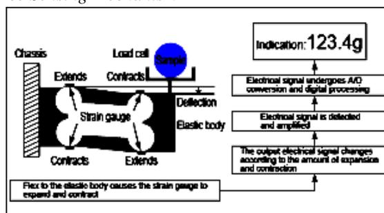
Fig 3: Load Cells in Force Sensing Structure [8]
