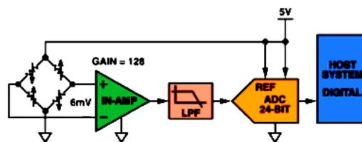
Fig 5: Filter for Dynamic Weighing System
