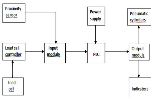
Fig 6: PLC based Automatic Weighing Control System [15]
