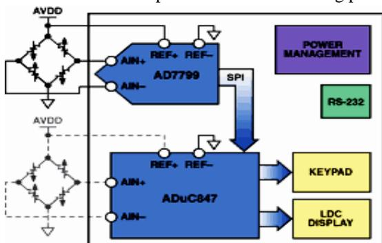
Fig 7: Weight Measurement System [27] Using Pic Microcontroller
