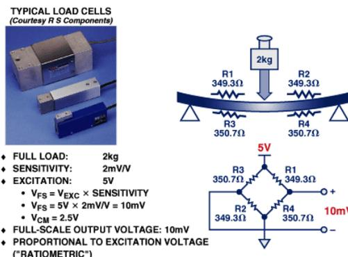
Fig 8: Typical Load Cell [28] with Sensitivity & Excitation
