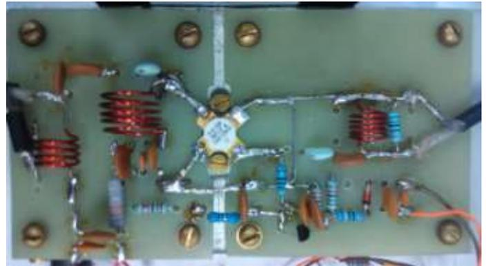
Figure 6a. Fabricated amplifier circuit
