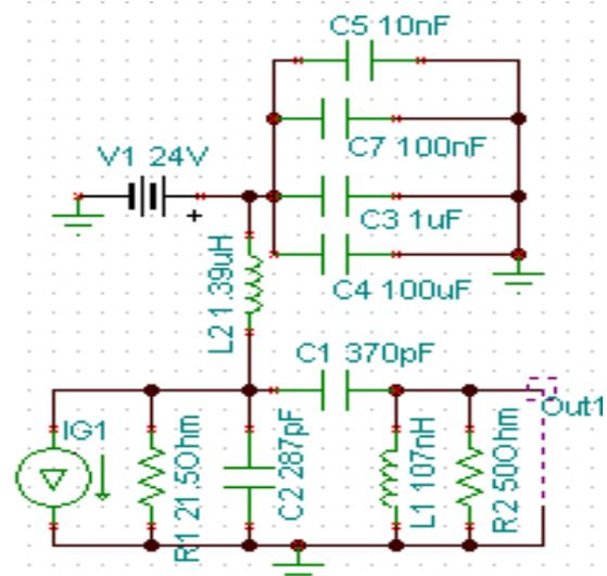
Figure 3. Simulated amplifier output circuit
