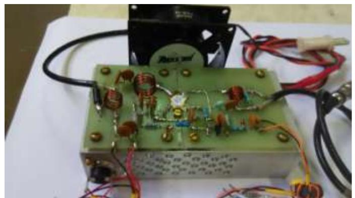
Figure 6b. Overall view of the amplifier module
