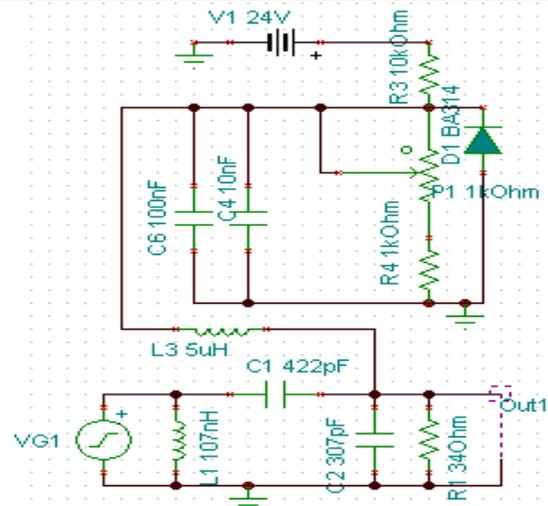
Figure 2. Simulated amplifier input circuit
