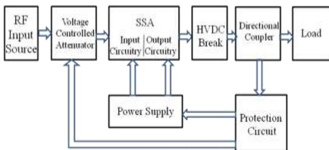
Figure 1. Block Diagram of Generalized Protection Scheme
