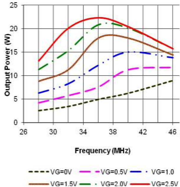
Figure 7. Solid State Power Amplifier response for Pi=200mW
