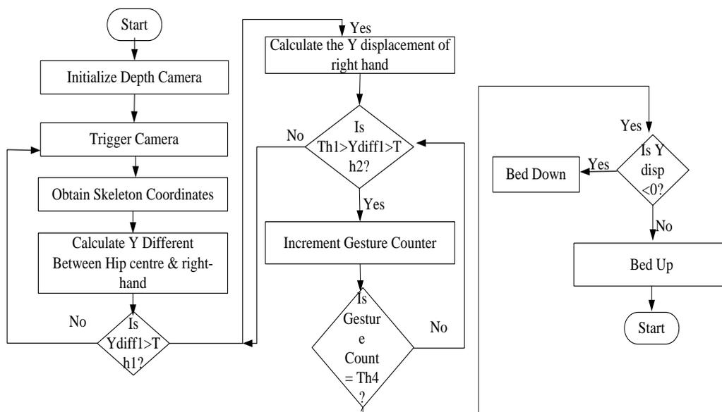
Figure.5. Flow Chart for Mode 1 Operation
