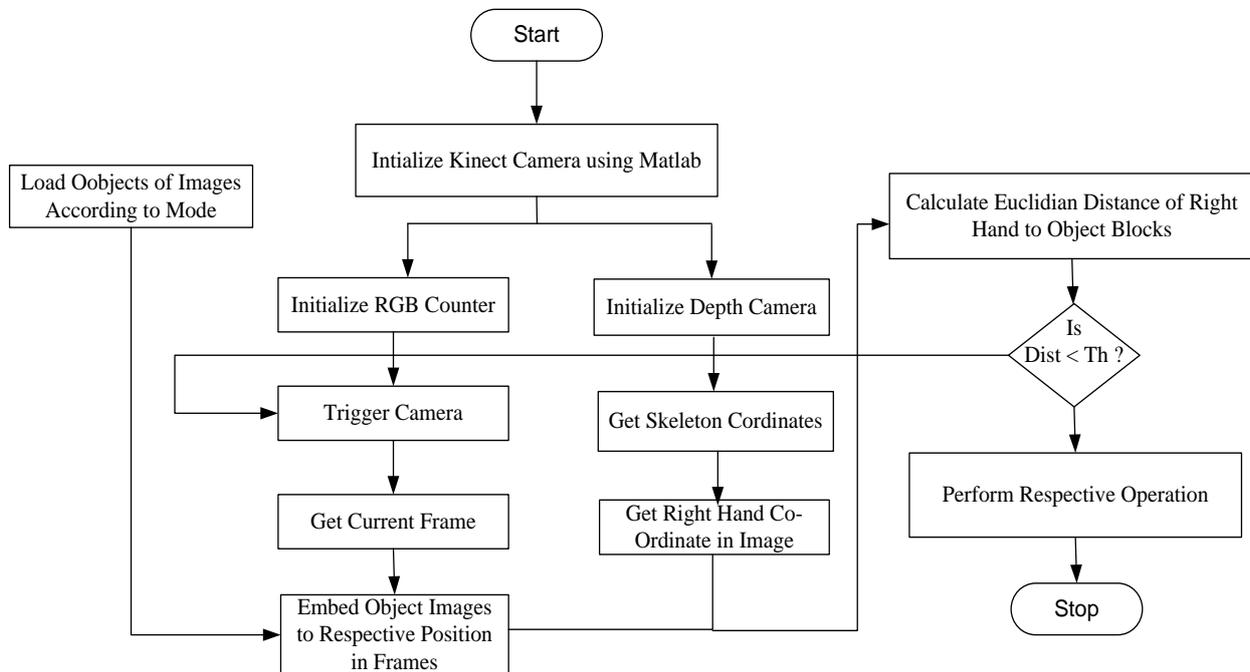
Figure 6. Flow Chart for the Mode 2 and Mode 3 Operations
