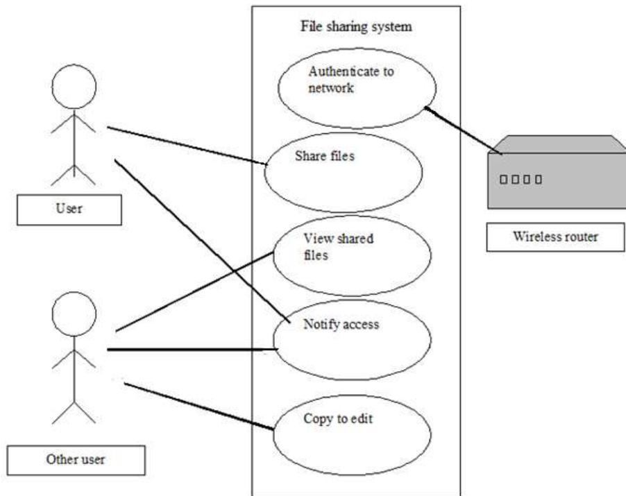
Figure 1 represents the Use case diagram for the system.
