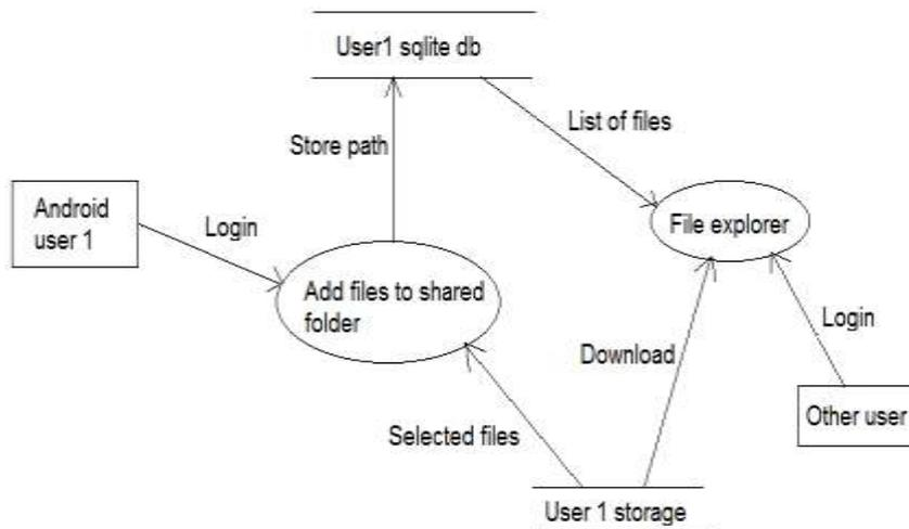
Figure 2 represents the level 1 DFD for the system.
