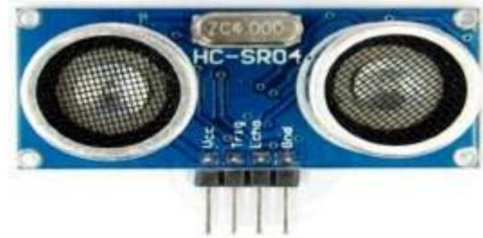
In Ultrasonic sensors, signal measurement is independent of material and color of obstacles. It works in all light conditions - bright, dark, glaring or dim. Suspended particles like dust, steam, smoke does not affect the measurements. HC-SR04 Ultrasonic Distance Sensor is a popular and low cost solution for non-contact distance measurement function. It is able to measure distances from 2cm to 400cm with an accuracy of about 3mm.
