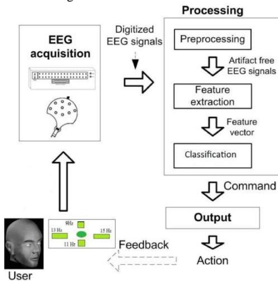
Figure 1. Conceptual block diagram of the proposed SSVEP based wheelchair control system.
