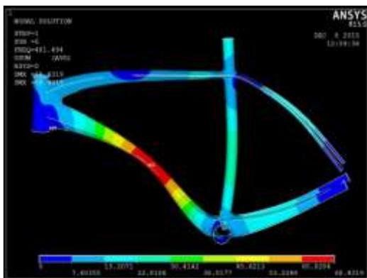
Figure 10: Frequency result at mode 5
