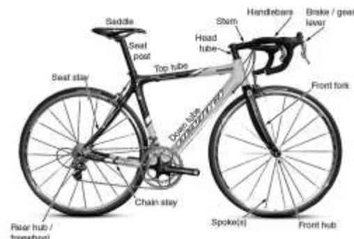
Figure.1: Bicycle frame and components
