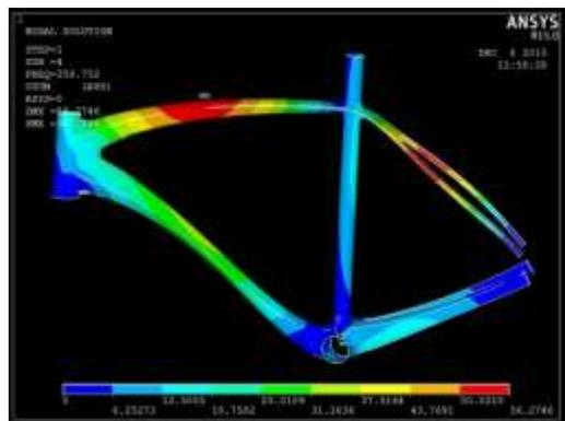
Figure 9: Frequency result at mode 4
