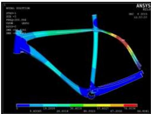
Figure 8: Frequency result at mode 3
