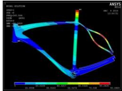
Figure 11: Frequency result at mode 6
