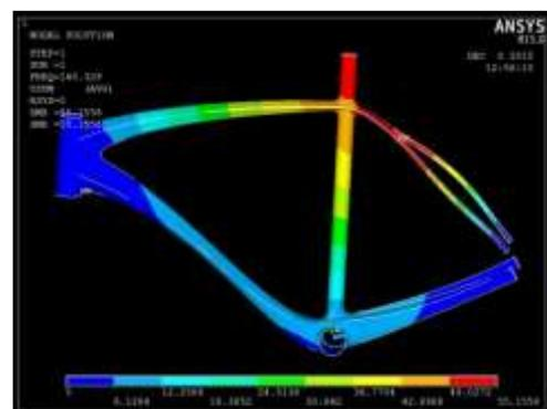
Figure 6: Frequency result at mode 1
