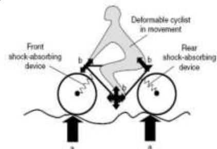
Figure 3: Forces transmitted to the frame
