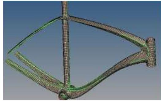
Figure 5: Meshed model with tetrahedral element
