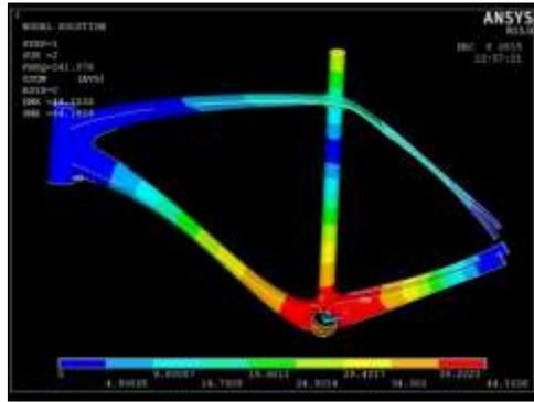
Figure 7: Frequency result at mode 2
