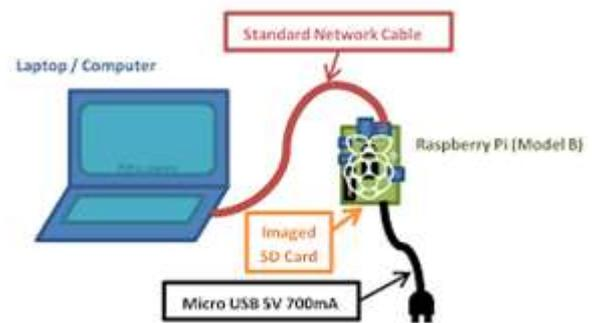
Fig. 5 Direct Laptop connection to Raspberry pi 2 Model B
