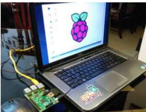
Fig. 4 Laptop connection to Raspberry Pi through router for Internet connection
