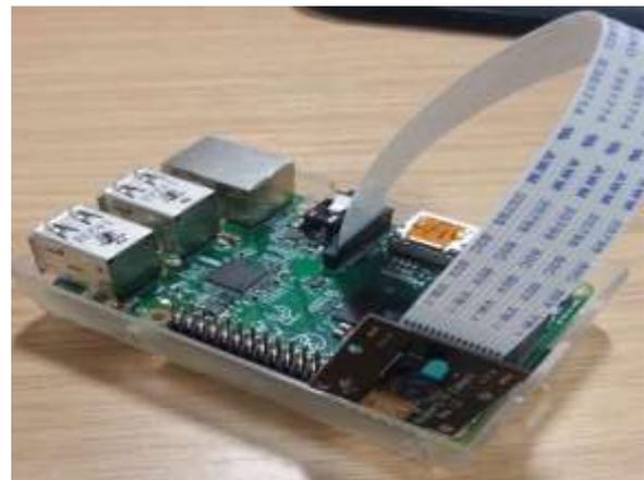
Fig. 3 Raspberry pi 2 Model B interfaced with Raspberry pi NOIR camera
