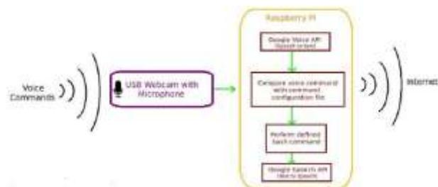
Figure 3. Working of Voicecommand software
