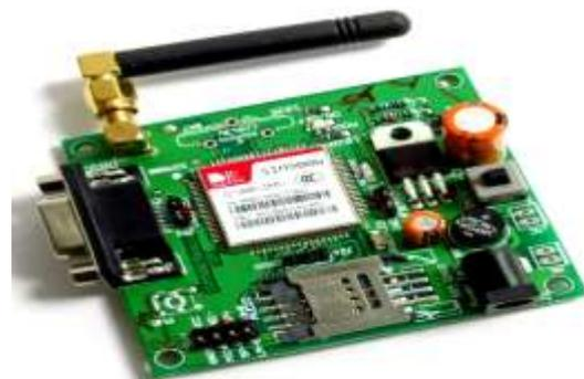
Fig.5: GSM SIM900A Modem
