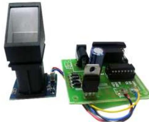
Fig.4: R305 Fingerprint Module
