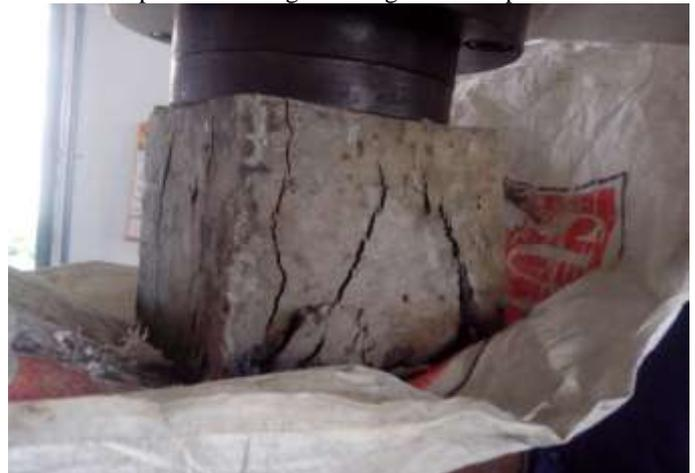
Flexural strength of the beam specimens are tested on UTM.
