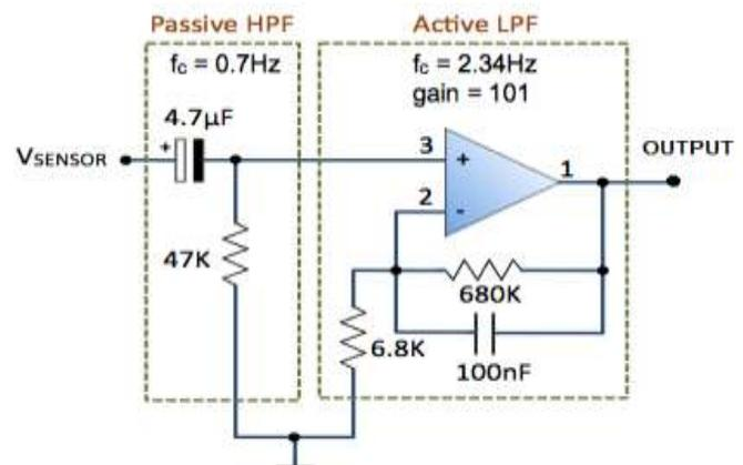
Figure 3: Band Pass Filter
