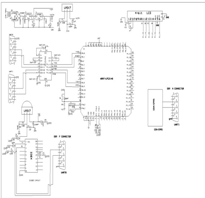
Fig.2.circuit diagram of server section
