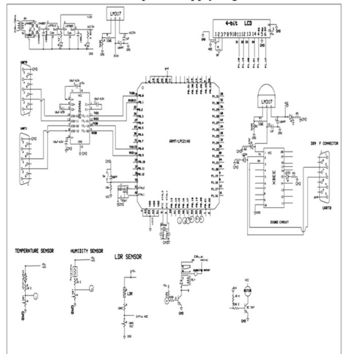
Fig.1.circuit diagram of Node section
