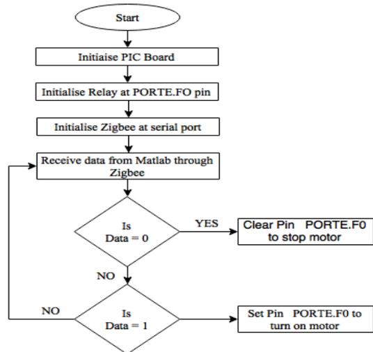
Third node consists of microcontroller PIC 16F877A along with Zigbee module, relay and AC motor. Command sent by controlling node is received by PIC microcontroller. As per command received, it will turn ON and OFF the motors in farm area.
