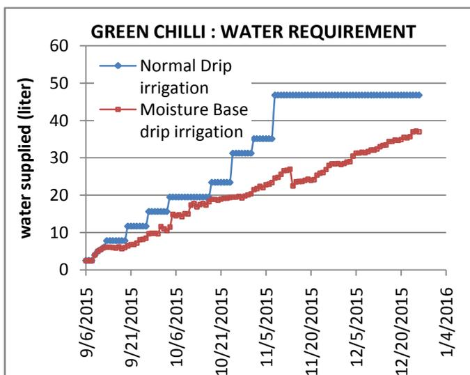
Figure 4: Water requirement of green chilly for normal and moisture based irrigation
