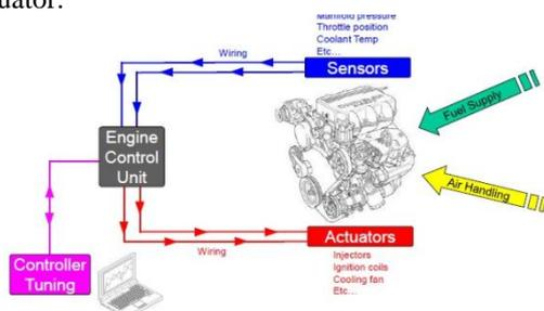
Figure 1: Working of Engine in closed loop
