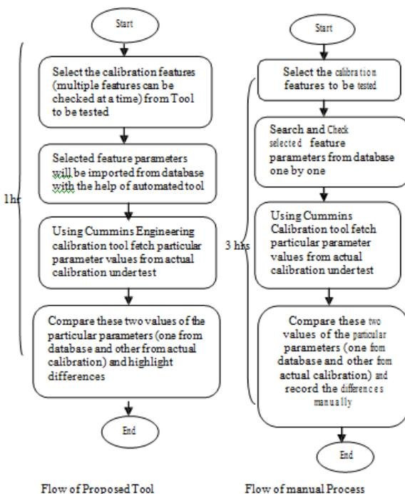
Figure2: Comparison between flow of automated tool and manual process and their time requirement
