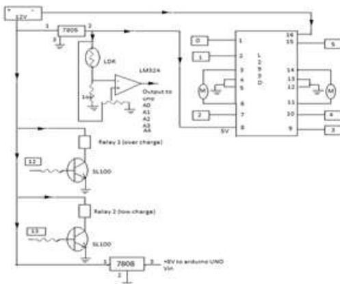
Fig (3):-LDR and motor circuit diagram
