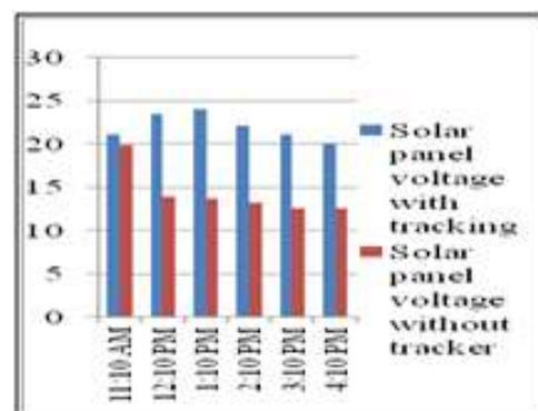
Fig(6):-Voltage without tracking system and with tracking
