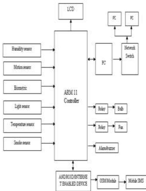
Fig 1: Block Diagram of the System
