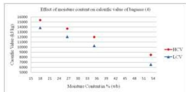
Fig.4. Effect of moisture content on calorific value of bagasse.
