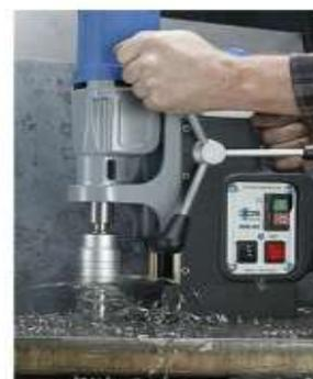
Fig 1.A magnetic core drill machine making hole.
