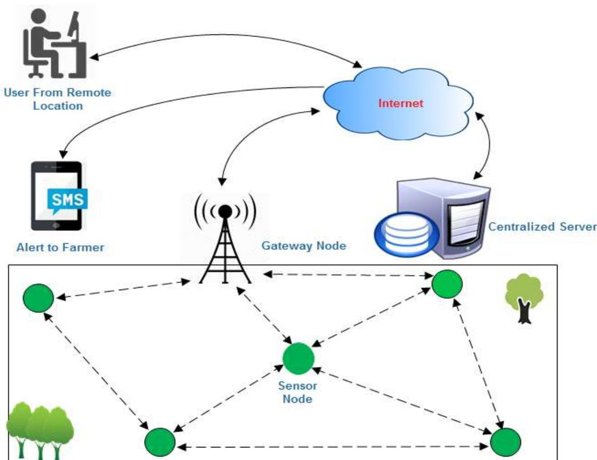
Figure 1. Wireless sensor network deployed on agriculture field.
