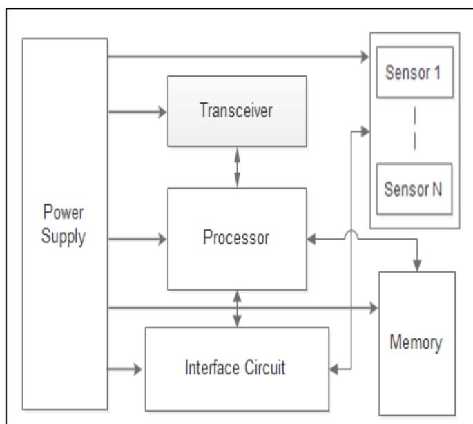
Figure 2 Structure of Sensor Node.
