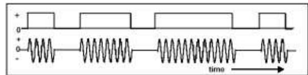
Fig. 2. Waveform ASK modulation
