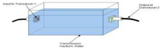
Fig. 6 Water as transmission medium and the ultrasonic transducer setup
