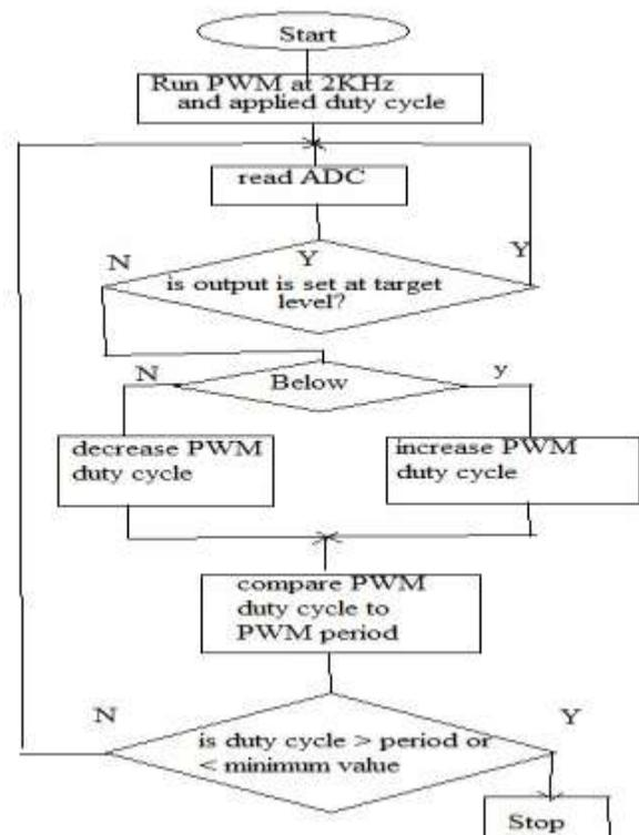
Fig.2 control algorithm
