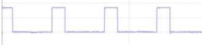
Fig.3 25% PWM duty cycle
