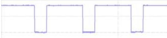
Fig.5 75% PWM duty cycle
