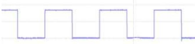
Fig.4 50% PWM duty cycle
