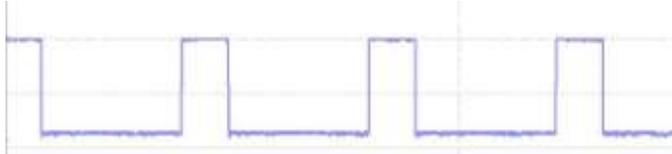
Fig.7 75% PWM duty cycle
