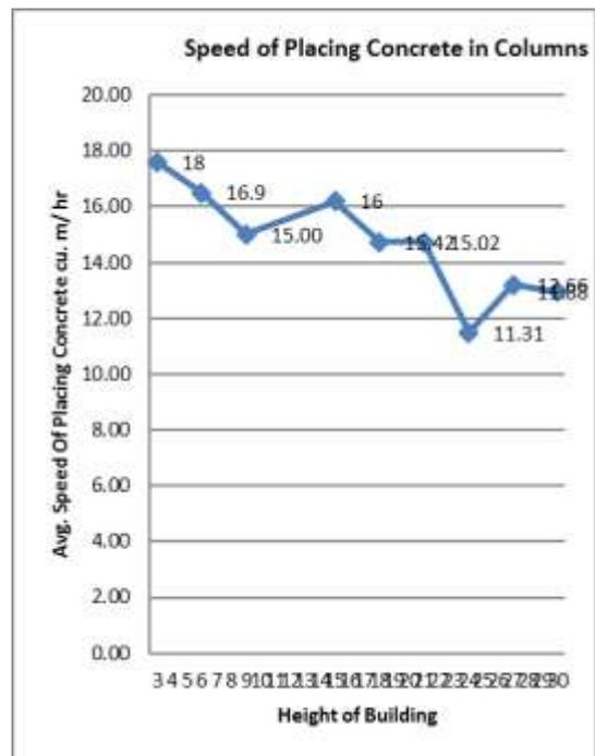
Fig. 1, Average Speed of Placing Concrete Vs Height of Building
