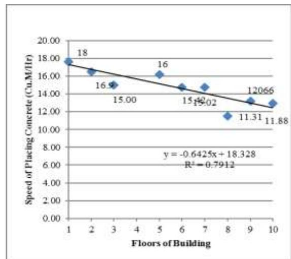
Fig.2, Speed of Placing Concrete Vs Number of Floors of Building
