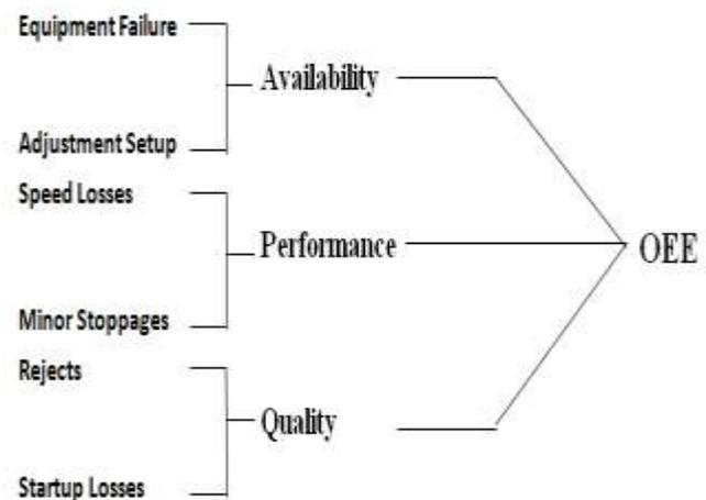
**Figure 2. Cascaded Model for Overall Equipment Effectiveness**
