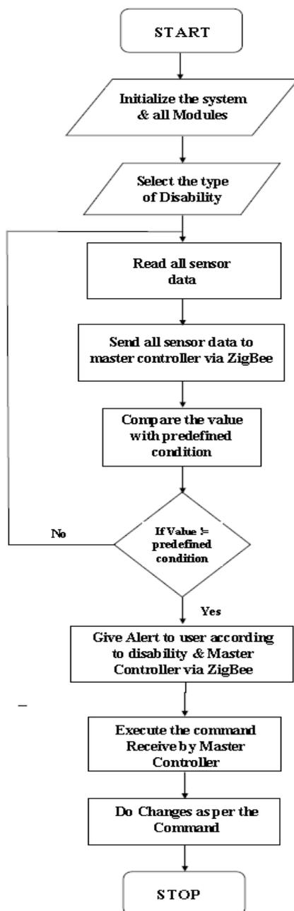
Figure 6 Flow Chart of System Working
