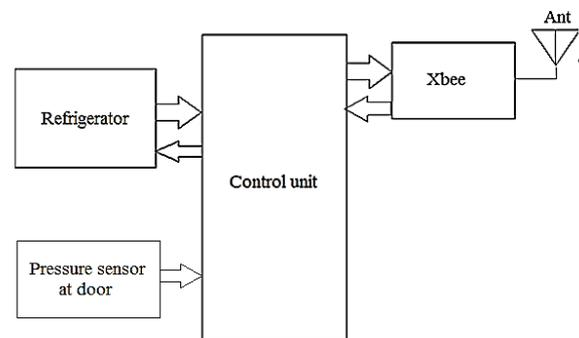
Figure 3 Refrigerator Control Unit
