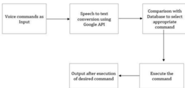
Fig. 1. Speech recognition block diagram
