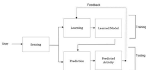
Fig. 2. Machine Learning block diagram
