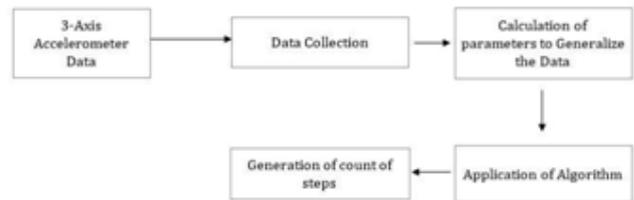
Fig. 3. Activity recognition block diagram
