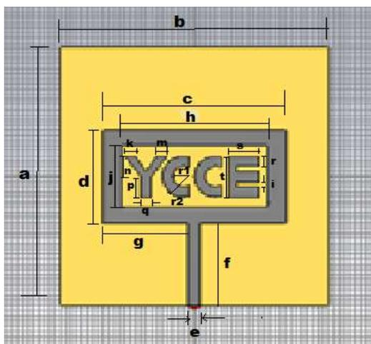
Figure 2: Patch antenna (Front view)
