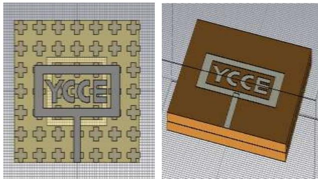
Figure 4: Patch antenna with EBG substrate (a) Top view and (b) Side view
