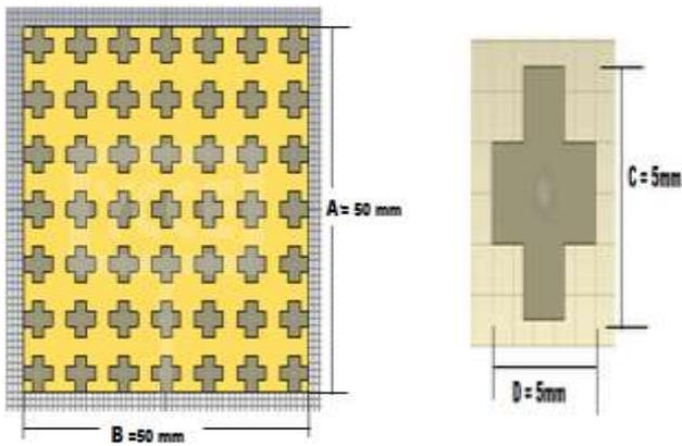
Figure 1: Design of EBG structure (a) Plus shape EBG substrate
