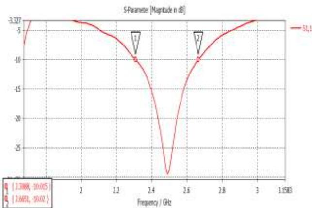
Figure 5: Simulated S-parameter result
