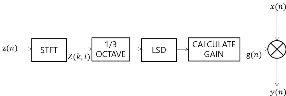
Figure 1. Block diagram of the proposed method.
