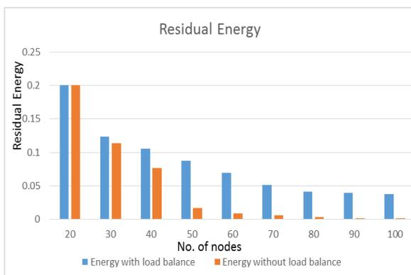
Fig. 2 Residual Energy of clustering with load balancing and clustering without load balancing in Joules
