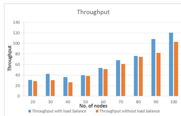
Fig. 3 Throughput of clustering with load balancing and clustering without load balancing in Bits/Sec
