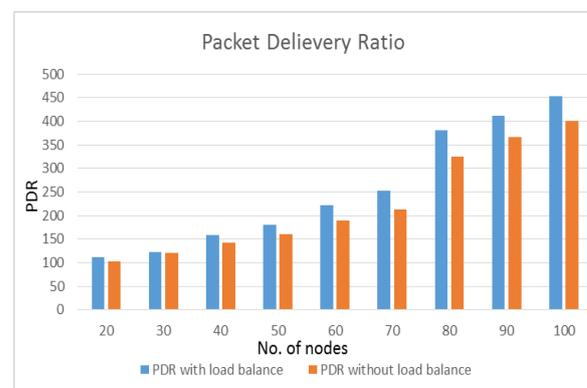
Fig. 4 PDR of clustering with load balancing and clustering without load balancing
