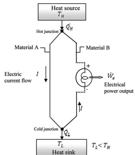
Fig. 3.Simple thermoelectric power generator operating based on Seebeck effect.
