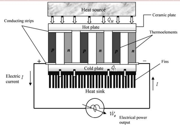
Fig 2- Thermoelectric effect
