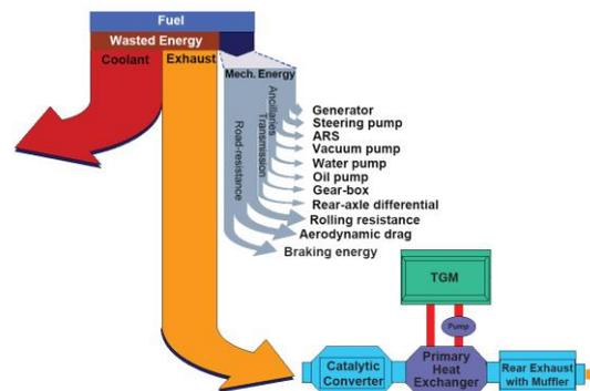
Fig. 1 Waste Heat from Internal Combustion Engine
