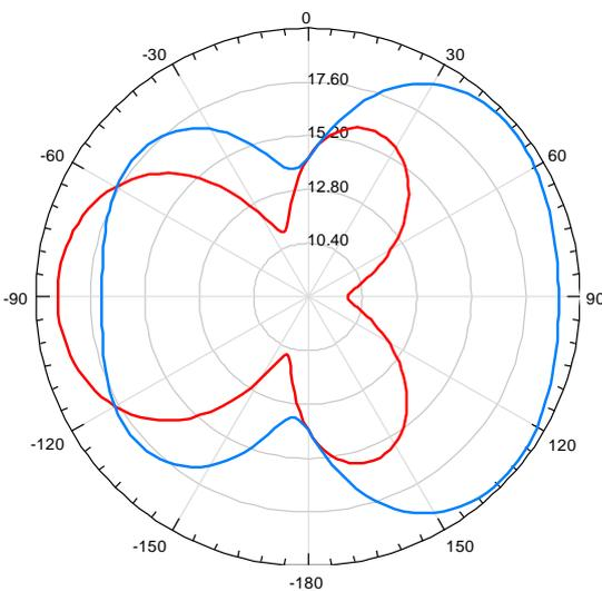
Figure 6. Radiation Pattern of proposed antenna at 9GHz
