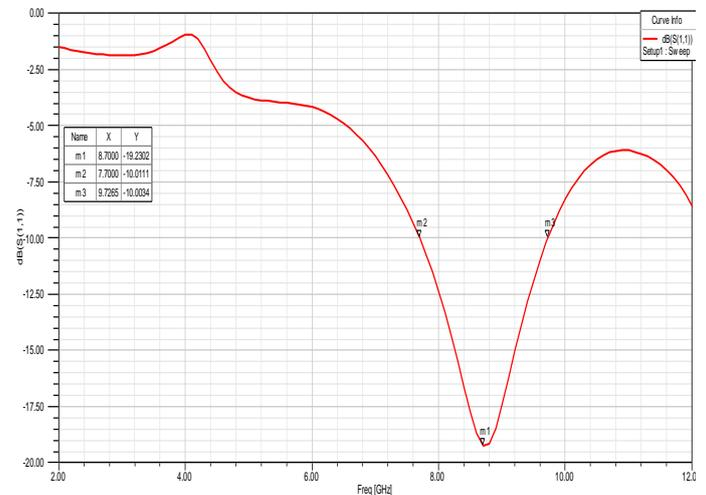
Figure 3. Simulated S11 characteristics of proposed antenna
