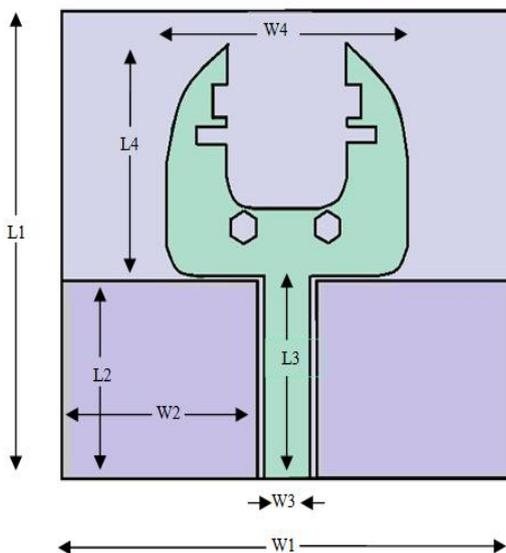
Figure 1. Geometry of the proposed antenna
