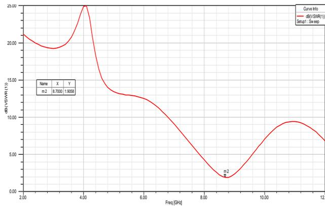
Figure 4. Simulated VSWR for the proposed antenna
