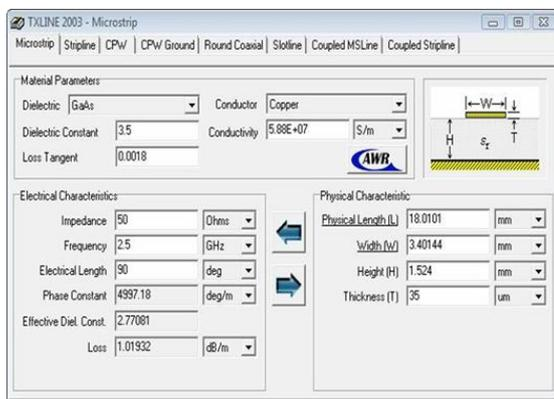
**Fig. 3.6 TXLine, used to convert between ideal elements and realistic ones.**
