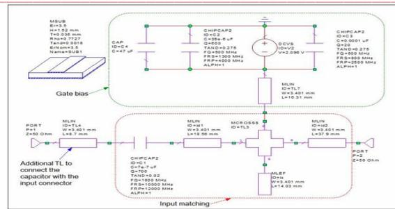
**Fig. 3.8 Input matching network with realistic ones.**
