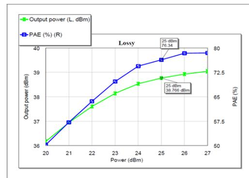
**Fig. 3.10 simulation results of class F power Amplifier with Realistic ones**
