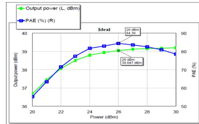
**Fig. 3.5 simulation results of class F power Amplifier with ideal components**
