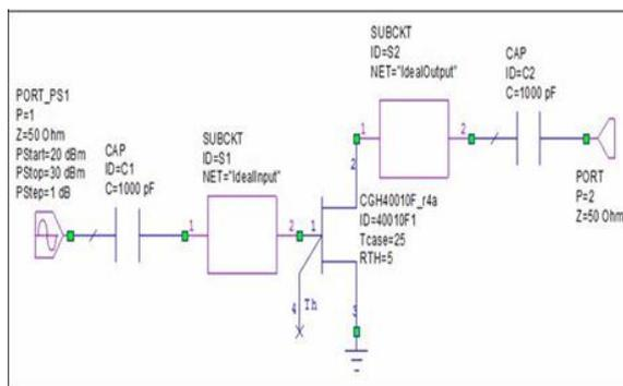
**Fig. 3.4 Power Amplifier circuit using ideal components.**
