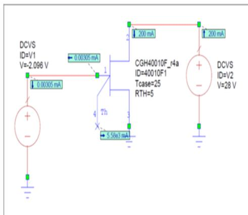
**Fig. 3.1 Circuit used to get gate bias voltage.**
