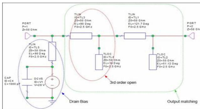
**Fig. 3.3 output matching network designed with ideal componenets**
