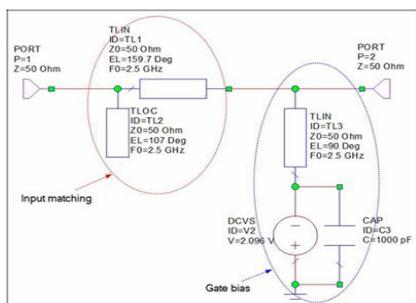
**Fig. 3.2 Input matching network designed with ideal componenets**
