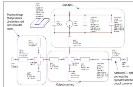
**Fig. 3.9 output matching network with realistic ones.**
