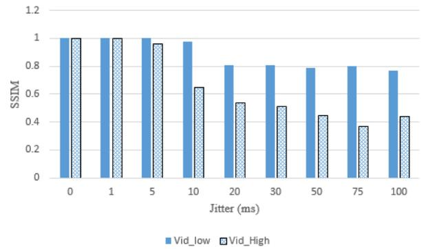
Figure 12. Effect of Jitter over SSIM index for low and high motion video
