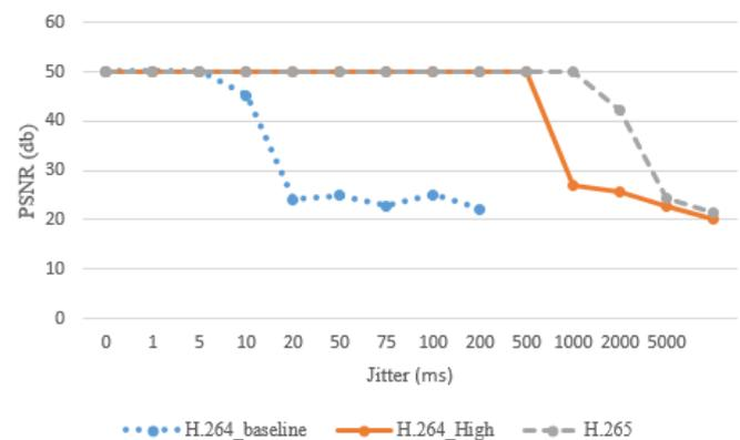
Figure 13. Effect of Jitter over video codec in terms of PSNR
