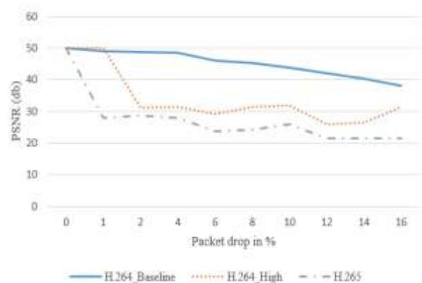
Figure 8. Packet drop Vs PSNR for different video codec
