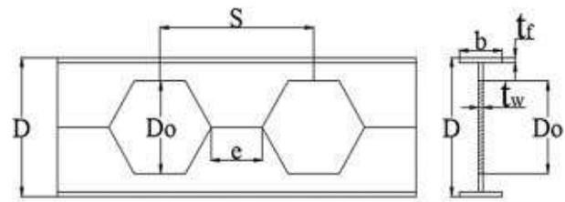
Figure2. Typical cross section of a beam
