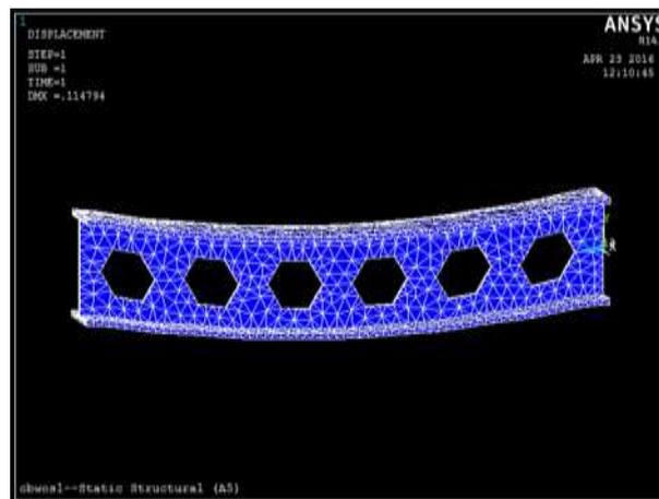
Figure 7. Ansys analyzed model without stiffeners
