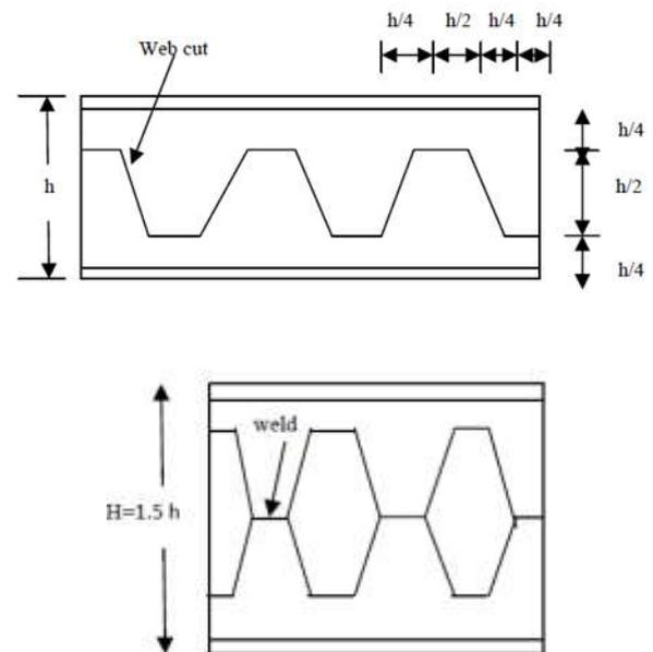
Figure 1. Fabrication of castellated beam with hexagonal openings
