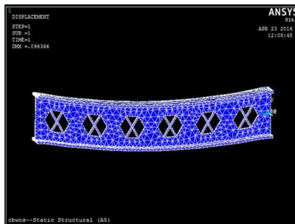
Figure 8. Ansys analyzed model with diagonal stiffeners
