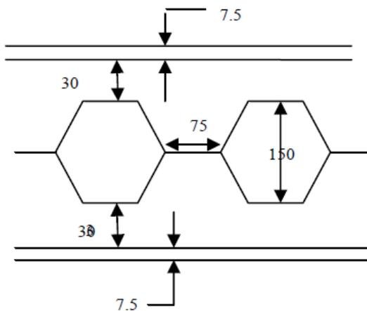
Figure 4. Design parameters of castellated beam
