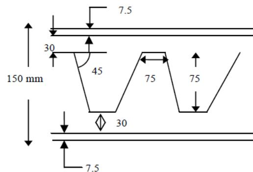
Figure 3. Design parameters of castellated beam
