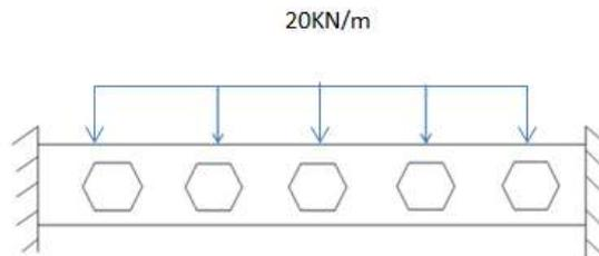
Figure 6. Fixed beam with uniformly distributed load
