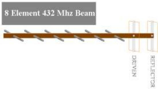
Figure-2: 8 element Quagi antenna
