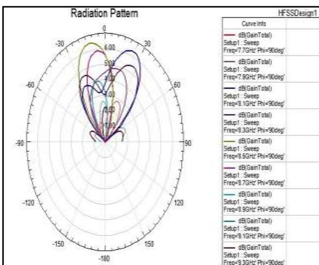
Figure 6: Far field radiation pattern of the antenna across the frequency band.
