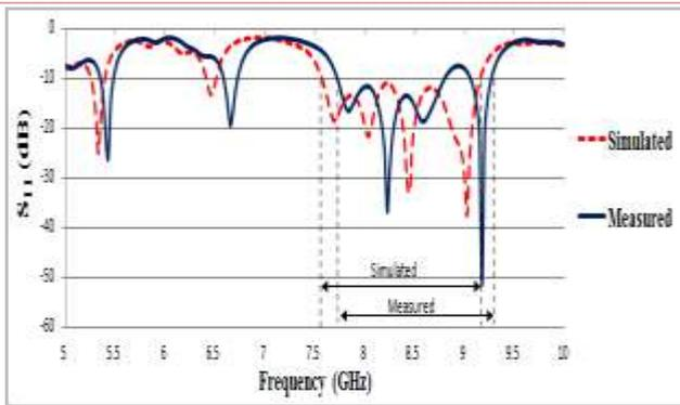
Figure 4: Return loss ( $S_{11}$ ) characteristic plot of the proposed antenna
