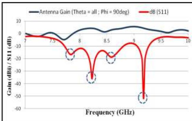
Figure 5: Antenna gain and return loss across frequency.
