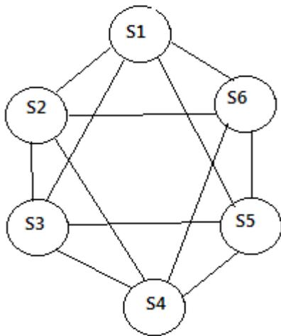
Fig 1: Circular Topology of Wsn With Six Sensor Nodes.
