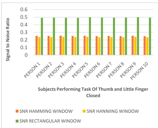
Fig.12 Signal to Noise Ratio comparison for thumb and little finger closed activity
