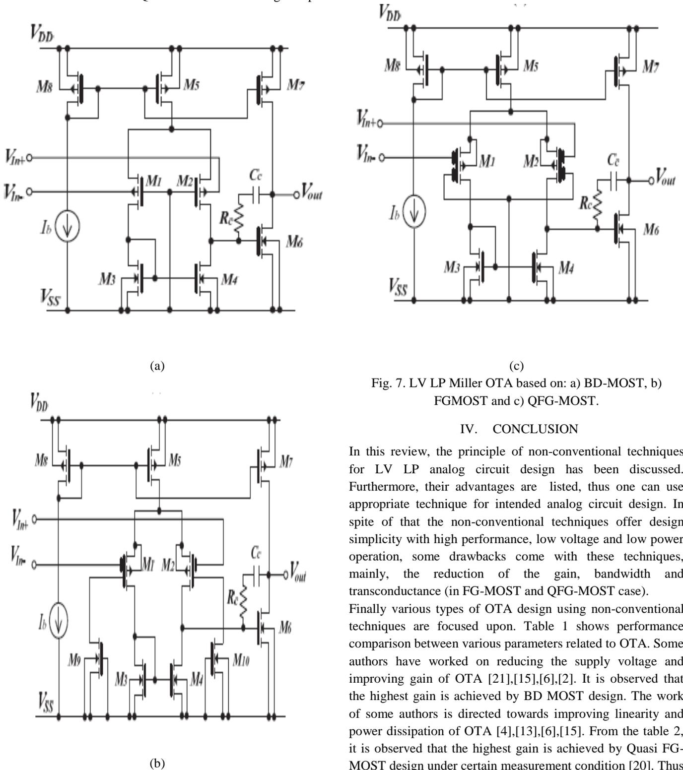
Fig. 7. LV LP Miller OTA based on: a) BD-MOST, b) FG-MOST and c) QFG-MOST.
