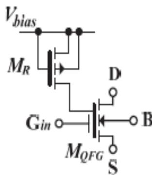
Fig. 5. One-input Quasi-Floating gate NMOST
