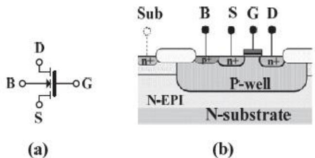
Fig. 1. Bulk-driven N-MOST: a) symbolic and b) cross-section.
