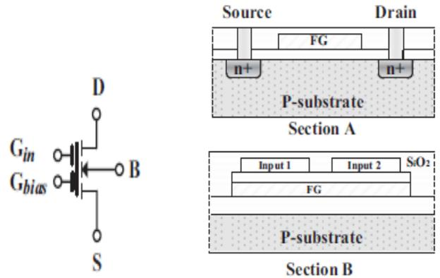
Fig.3. Two-input floating gate NMOST: a) symbolic, b) cross-sectional views.
