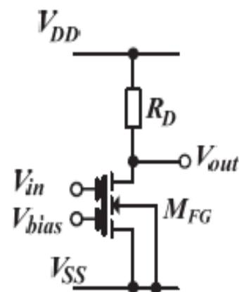
Fig. 4. Floating-gate MOST: common source amplifier
