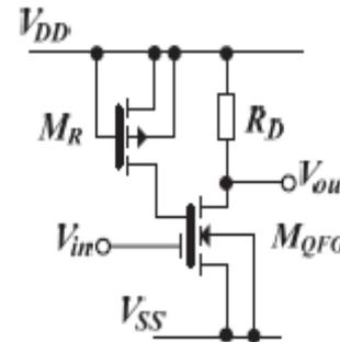
Fig. 6. Quasi-Floating gate MOST: common source amplifier with single input terminal
