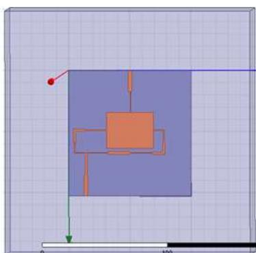
Figure 1. Patch antenna with power divider
