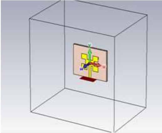
Figure 6 .First iteration of Koch Fractal loop antenna
