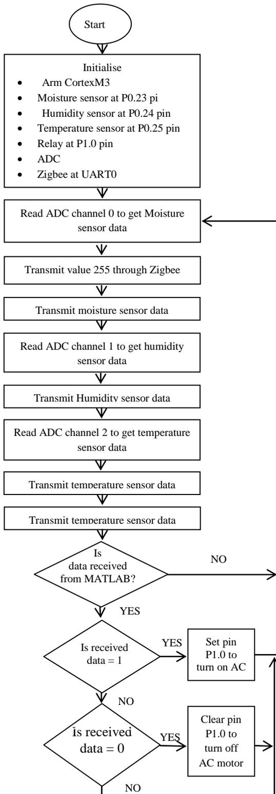
Figure 3: Algorithm for ARM Cortex M3
