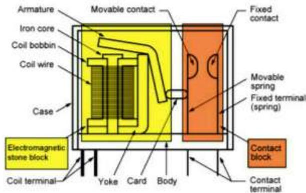
Fig.5:Cross Section Of Relay
