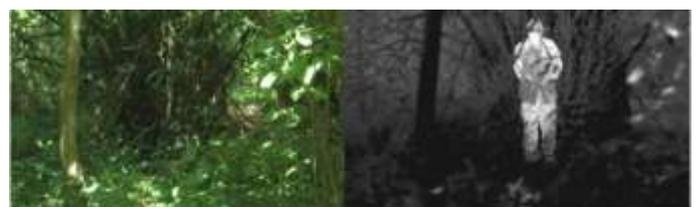
Fig.16: View of same image by normal camera and thermal image camera [24]
