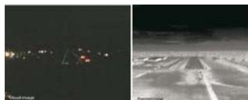
Fig. 20: View of flight runway using visual image and Thermal camera Image [32]
