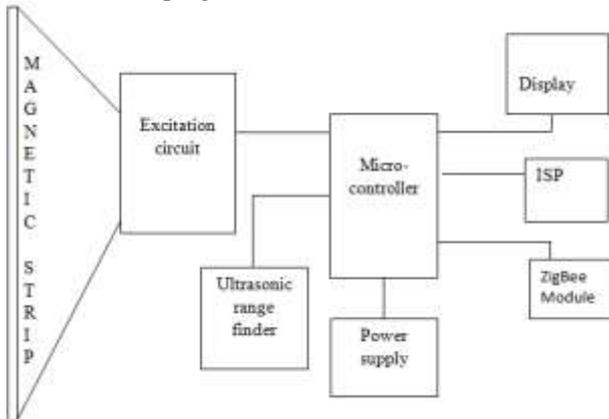
Fig. 9: Block diagram of anti-collision system [12]
