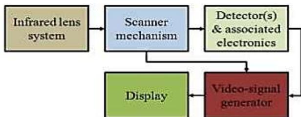
Fig. 18: Block diagram of signal routing in infrared camera [28]
