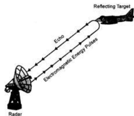
Fig. 1: Schematic diagram of radar operation [3]
