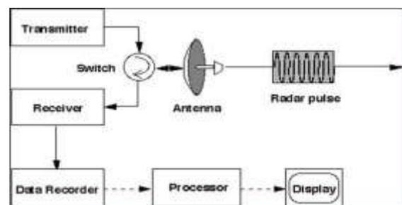
Fig. 2: Block diagram of radar circuit [4]
