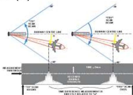
Fig. 8: Microwave landing system coverage [11]
