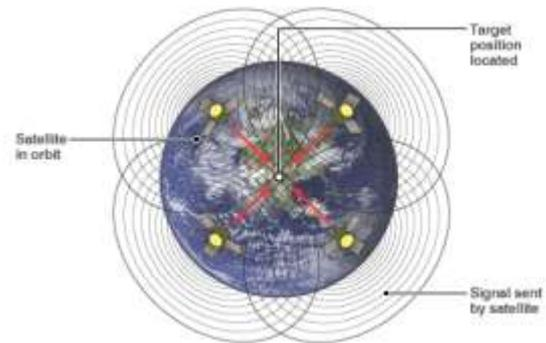
Fig.11: Schematic diagram of GPS operating principle[15]
