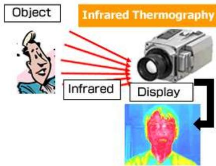
Fig. 17: Schematic diagram of operating process of infrared thermography [27]
