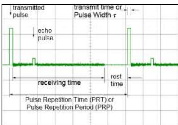
Fig. 4: Transmitter and receiver synchronization in basic radar [5]
