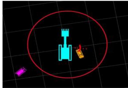
**Fig. 5:** Radar assisted aerial view of other vehicles position for a shovel [8]
