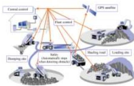
Fig. 13: Schematic diagram of GPS application in opencast mine [18]
