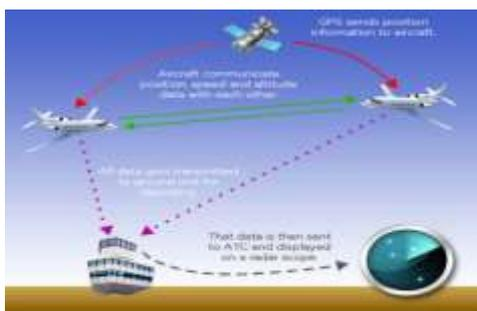
Fig.14: Schematic diagram of operating procedure of ADS-B system [21]
