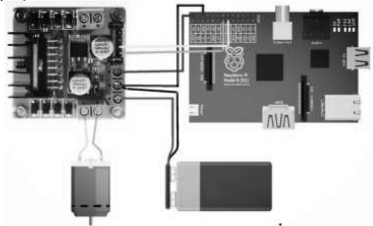
Figure 3 Connection of Raspberry Pi with L298N motor driver[9]
