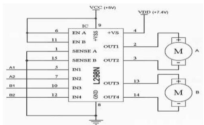
Figure 4 Circuit Diagram of Connection of motor driver with motors[10]
