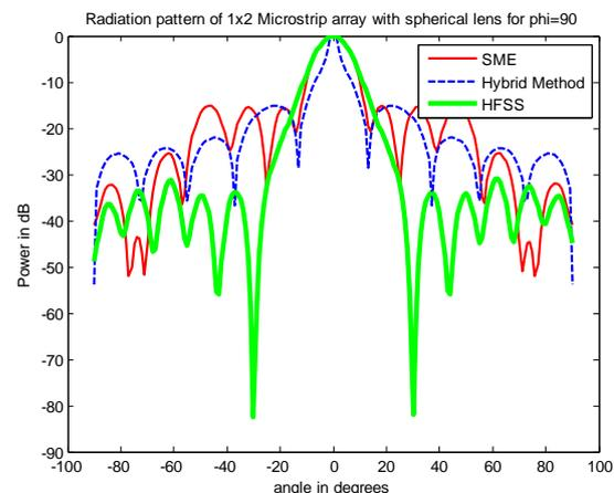
Fig4: Radiation pattern of 1x2 Patch array with Spherical lens at 6GHz for phi=90
