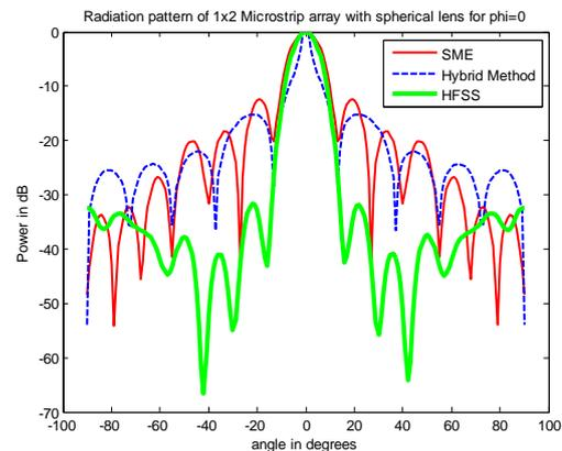
Fig3: Radiation pattern of 1x2 Patch array with Spherical lens at 6GHz for phi=0
