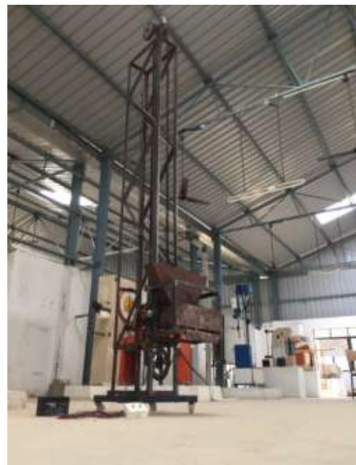
Figure 2 : Automatic Wall Plastering Machine
