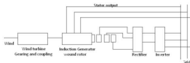
**Block Diagram double output of IGWR**
